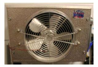
Figure 2.8 The evaporator unit fan
