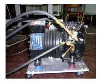
Figure 2.3 System compressor
